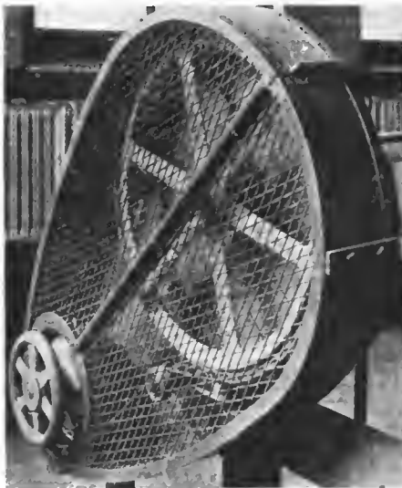
Above is illustrated the type of expanded metal and sheet iron guard employed in the Republic factory for sprocket and chain drives of the sort illustrated
